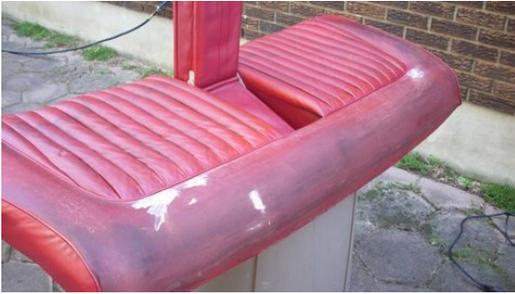
old dye removed and crack filler
