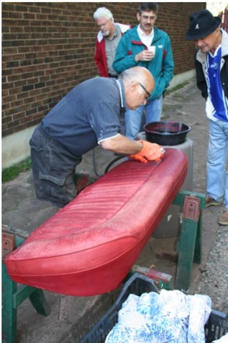
Once the seat has been cleaned and the dye removed then a number of liberal coatings of leatherique rejuvenating oil is applied to soften the leather. 5 Coats a few days apart is optimum. Leatherique recommends that when using their product the use of Pristine Clean precede the use of the rejuvenating oil to remove embedded dirt and previous layers of dye. These leatherique products are water based.
