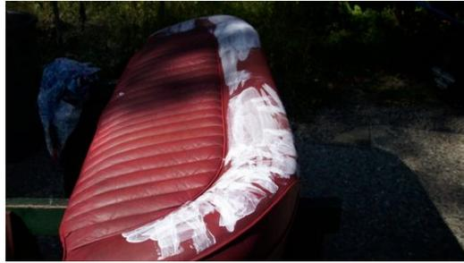
old dye removed and crack filler
